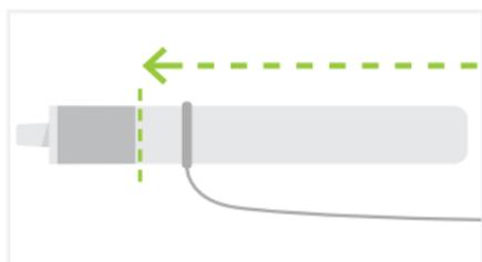
Slide the strap ring down the handle to just below the flexible joint.
