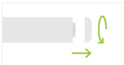
Swivel the end cap counter-clockwise to unlock and pull to remove.
