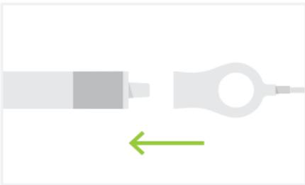
Plug the leveling handle into the ring-shaped end of the charging connector with the magnets.
