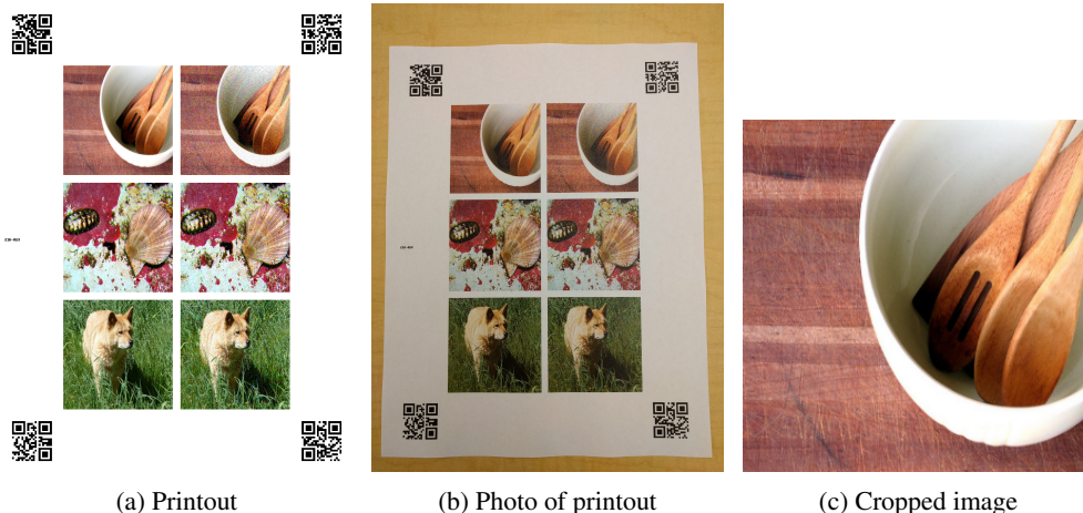
Figure 4: Experimental setup: (a) generated printout which contains pairs of clean and adversarial images, as well as QR codes to help automatic cropping; (b) photo of the printout made by a cellphone camera; (c) automatically cropped image from the photo.
