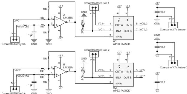
Figure 5. Current-drive circuitry for two voice coil actuators.
