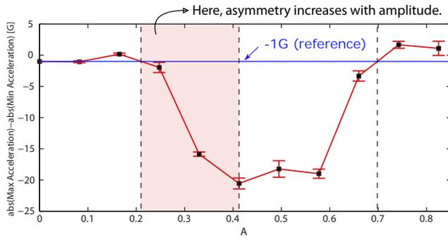
Figure 9. Acceleration asymmetry vs. Amplitude of Current.
