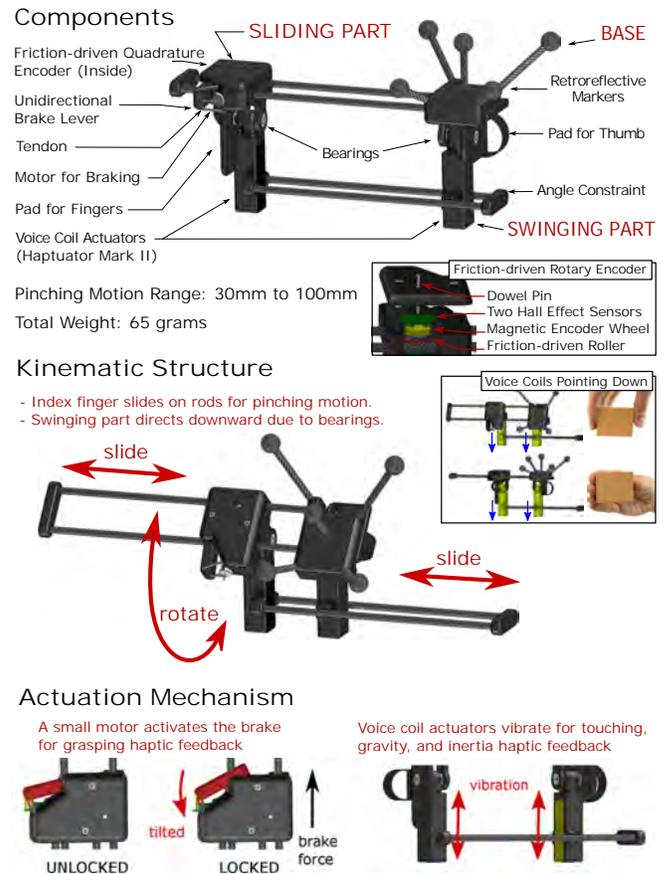
Figure 3. Overall mechanical structure and actuation mechanism.
