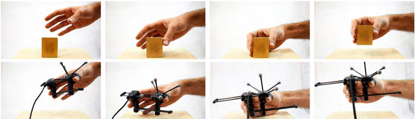
Figure 1. *Grability* is a novel, unified design based on the combination of vibrotactile feedback, uni-directional brakes, and asymmetric skin stretch. The gripper-style haptic device can simulate grasping motions with a real object (top), in Virtual Reality (bottom). Gravity provides vibrotactile feedback during contact, high stiffness force feedback during grasping, and weight force feedback during lifting.
