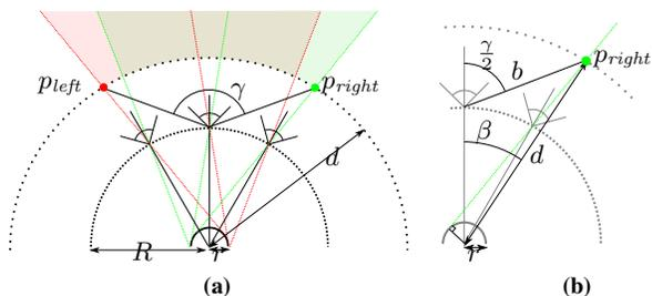
**Figure 9:** (a) To successfully stitch all points with distances of at least  $d$  from the rig center, the central camera must observe all points in the shaded regions (red for right eye and green for left eye). The extreme points  $p_{left}$  and  $p_{right}$  constrain the camera's field of view to be at least  $\gamma$ . (b) Here we visualize the intermediate values used when defining  $\gamma$  in (6).
