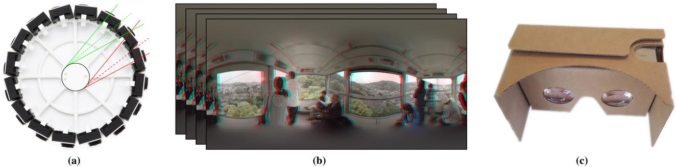
**Figure 1:** The Jump system produces omnidirectional stereo (ODS) video. (a) The multi-camera rig with the ODS viewing circle overlaid and three rays for the left (green) and right (red) stitches. Solid rays pass through a camera and can be sampled directly. Dashed rays are sampled from interpolated views. (b) A stitched ODS video generated from 16 input videos, shown in anaglyphic stereo here. (c) A VR headset in which the video can be viewed.
