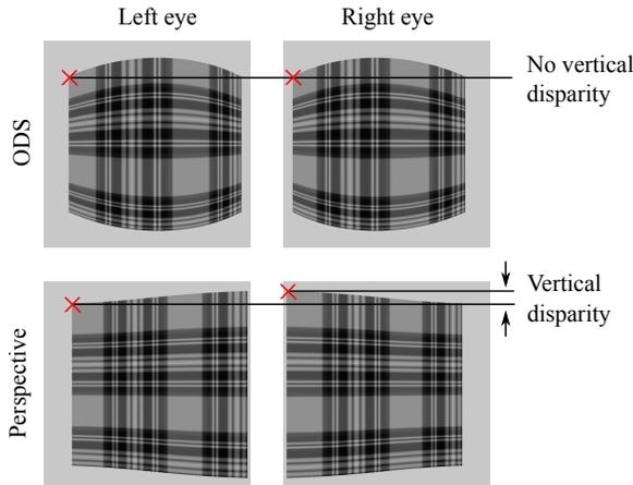
**Figure 3:** A synthesized, textured square imaged by the ODS projection and then projected to perspective. The images have an interpupillary distance of 6cm and about 100° FOV. The square has been placed at the unusually close distance of 30cm to exaggerate the vertical parallax for the figure.
