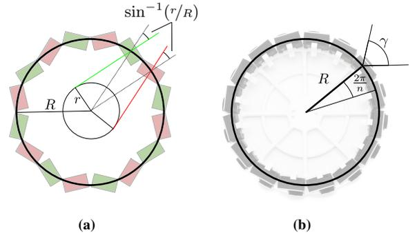
**Figure 8:** Sketch of a tangential (left) and radial (right) layout. (a) In the tangential case, the cameras align with the ODS left/right rays by rotating  $\pm \sin^{-1}(r/R)$  w.r.t. the radial direction. (b) The radial rig geometry is fully defined by its radius  $R$ , number of cameras  $n$ , and the horizontal field of view  $\gamma$  of the cameras.
