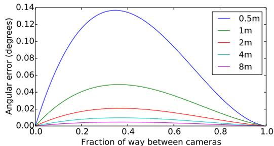
**Figure 14:** The error introduced, for points at various distances from the rig center, by using the approximation in Eq. 16 rather than synthesizing intermediate views explicitly and generating an ODS stitch from those.
