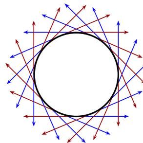
**Figure 2:** The omnidirectional stereo (ODS) projection which captures stereo views in all directions by sampling rays tangential to a viewing circle. Red and blue rays comprise left and right eyes respectively.
