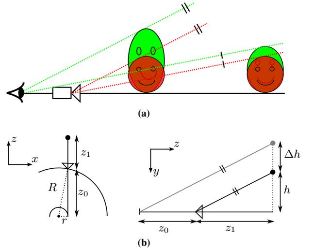
**Figure 7:** (a) Vertical distortion caused by capturing with cameras which lie on a larger circle than the ODS viewing circle. The red faces are viewed by a camera. When the parallel rays are used for rendering from a viewpoint behind the camera this leads to the vertically stretched green faces. (b) Top and side views of this distortion being applied to a point.
