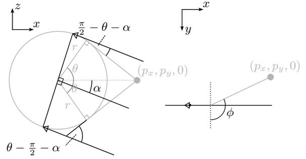
**Figure 4:** Top and side views of a point being projected into ODS space (greyed out) and the angles of the rays that view it with respect to two perspective views for a horizontal view rotated  $\alpha$  from the point.
