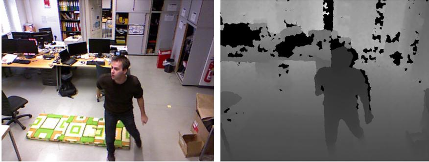
**Fig. 4** RGB camera image and its corresponding depth image.
