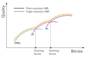
**Figure 1.** The rate-quality performance of single resolution ABR streams are illustrated by the dashed lines. With multi-resolution ABR streaming, better rate-quality performance can be achieved, which is illustrated by the solid line. The cross-over points between these rate-quality curves determine the optimal bit rate range for switching between resolutions.
