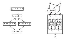
Fig. 1. CFG (left) and RVSDG (right) representations of the same function, computing x-y if x>y and y-x otherwise.
