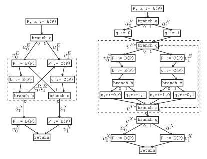
Fig. 3. Restructuring of loop control flow. Left: Unstructured CFG (loop with two entry and exit paths). The vertices within the dashed box form an SCC. Right: Restructuring the left CFG. The subgraph in the dashed box corresponds to the loop body and is treated as if it were collapsed into a single vertex from the point of view of the outer graph. The dotted arc is the single repetition arc.
