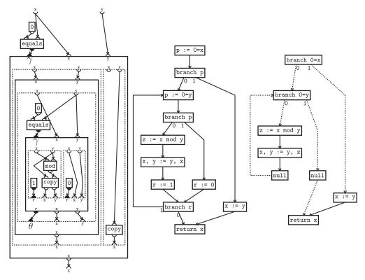
Fig. 2. Euclid's algorithm in different representations. Left: Representation of the algorithm as RVSDG. Center: CFG generated from RVSDG on the left by SCFR. Right: CFG recovered from RVSDG on the left by PCFR. The solid arcs are generated in the first pass by PREDICATIVECONTROLFLOWPREPARE; the dotted arcs are generated in the second pass by PREDICATIVECONTROLFLOWFINISH.
