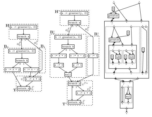
Fig. 4. Restructuring of branch control flow. Left: Unstructured CFG (inconsistent selection paths). Middle: Restructuring the left CFG. Right: The RVSDG equivalent to the CFGs to the left.
