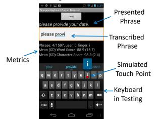
Figure 3. The UI of Keyboard Output Receiver as Octopus *remulates* the phrase "please provide your date." The red dot marks a simulated touch point.
