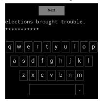
Figure 5. The WOZ keyboard we used to collect data for evaluating STKs. The keyboard design aims to capture fundamental text entry behavior.
