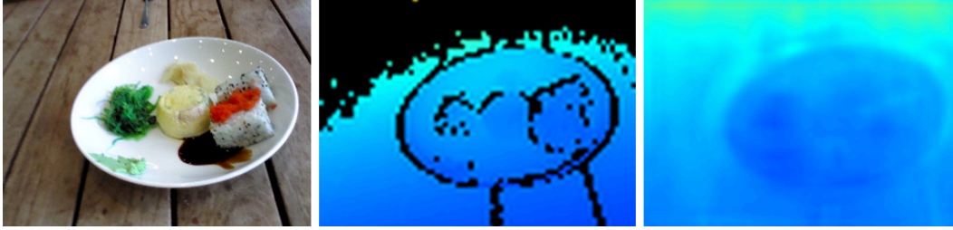
Figure 6. (a) An image from the GFood-3d test set. (b) Depth recorded from RealSense RGBD sensor. (c) Depth predicted by CNN.
