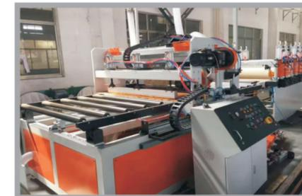
**SPC Flooring One Step Extrusion Line****SPC 地板一步法挤出生产线****SPC Flooring One Step Extrusion Line** SPC 地板一步法挤出生产线
