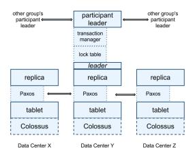
Figure 2: Spanserver software stack.
