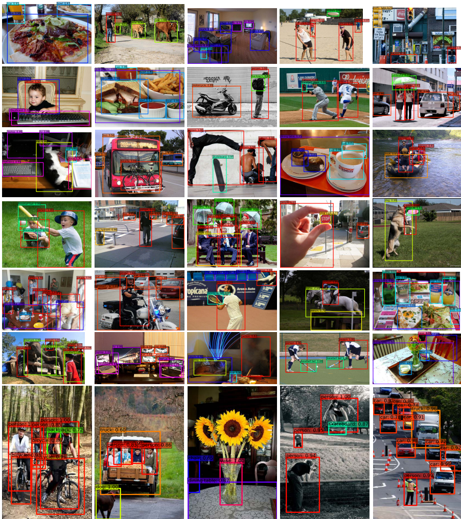
Fig. 5: Detection examples on MS COCO test-dev with SSD500 model. We show detections with scores higher than 0.6. Each color corresponds to an object category.
