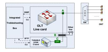
Fig. 6. Integrated Troubleshooting Box (ITB) and connectivity details
