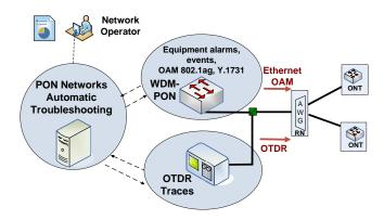
Fig. 1. Integrated Troubleshooting Box (ITB): Architecture
