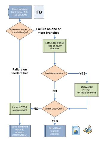
Fig. 7. The troubleshooting algorithm running on the ITB.
