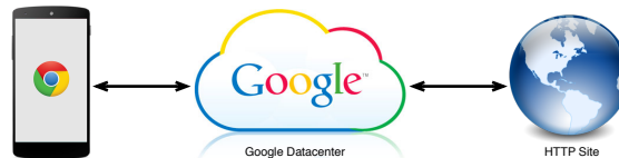
Figure 1: Flywheel sits between devices and origins, automatically optimizing HTTP page loads.
