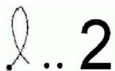
Figure 6 shows how to type in the cursive 'L' followed by the Dot and the number '2' to put the Palm in 'Console Mode'
