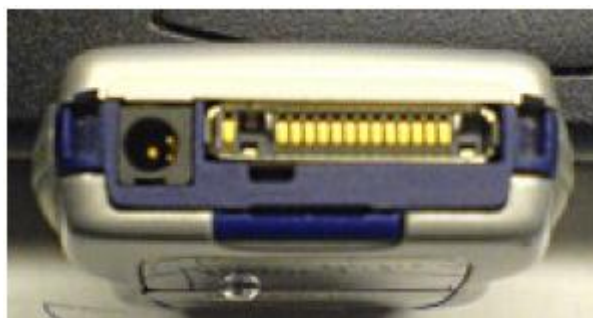
Figure 8: Nokia 3220 Fbus connections (Harrington 2007).
