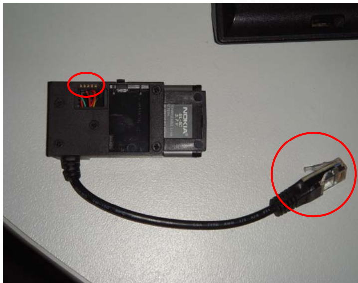
Figure 7: Connectors on the UFS3 cable for Nokia 6600
