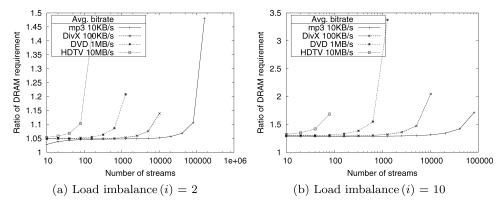
Fig. 17. Improvement in DRAM requirement of the integrated over the partitioned configuration for different load imbalance values.
