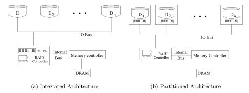
Fig. 1. Extended storage hardware architectures, integrated and partitioned.
