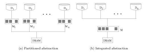
Fig. 2. Logical hardware abstractions corresponding to the hardware architectures in Figure 1.
