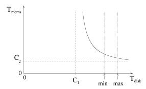
Fig. 9.  $T_{mems}$  as a function of  $T_{disk}$ . DRAM buffering can be reduced by increasing  $T_{disk}$ .
