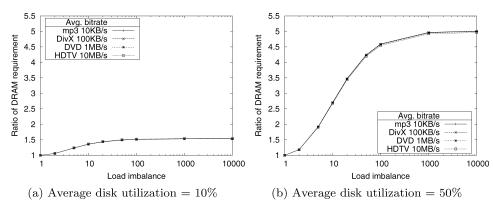
Fig. 14. Improvement in DRAM requirement of the integrated over the partitioned configuration for different average disk utilization values.
