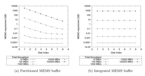
Fig. 19. MEMS requirement for individual disks for h = 1000.
