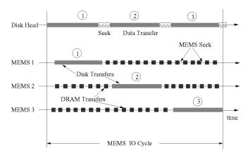
Fig. 5. IO Scheduling for a MEMS bank.
