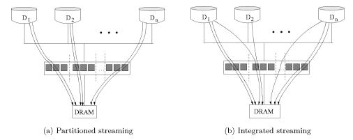
Fig. 6. The partitioned and integrated MEMS buffer schemes.
