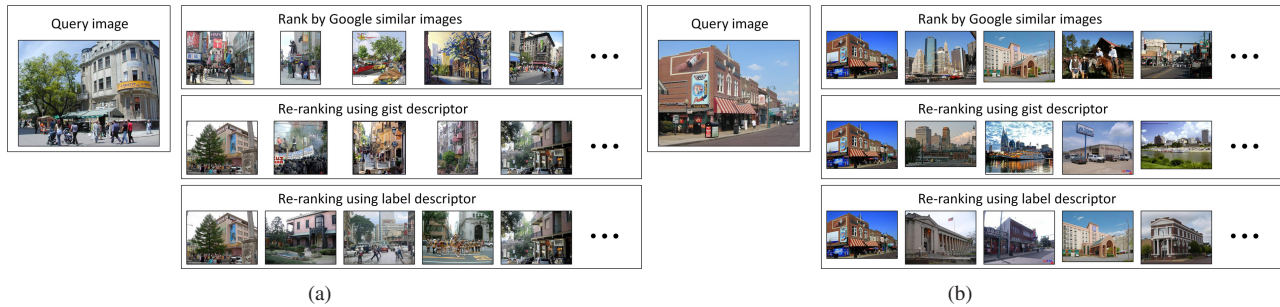
Figure 7: Application of the label descriptor to reranking Google similar images. Google similar image returns about 400 images for a query image. We run both the label-based descriptor and the Gist descriptor to rerank these images. Note that the label descriptor can find more semantically similar images than the Gist descriptor which only finds very similar images.
