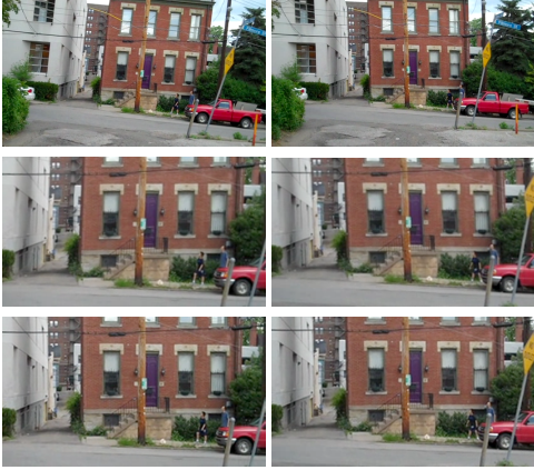
Figure 10: Reducing rolling shutter by our wobble suppression technique. Shown are the result for two frames 1/3 second apart. Top row: Original frames m (left) and m + 1 (right). Middle row: Stabilization result without wobble suppression. Bottom Row: Stabilization with wobble suppression. Notice, how wobble suppression successfully removes the remaining skew caused by rolling shutter. (The yellow traffic sign is tilted in reality.)
